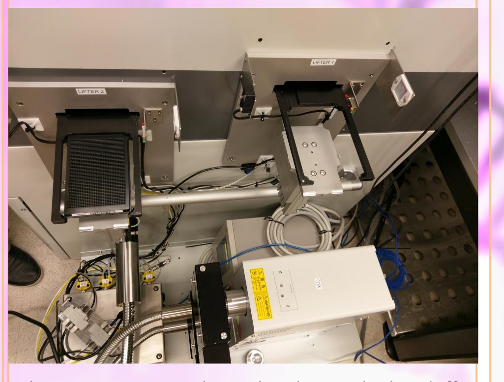
Integration of the IonField Tip Charger presented the greatest challenge as the FDSS wasn't designed with any empty bays in its tip/pin tool wash area. The pin tool blotter station was deemed the best location. Initial trial revealed that a mount with a very fine positional resolution would be necessary, and the X-Y gantry robot too low to clear the Tip Charger when in the pin tool pickup position.
