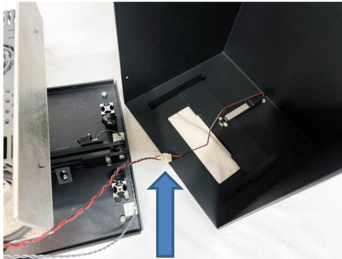
*Figure 66 – Plasma Module – Interior of Lid, Location of Door Actuator Plug*
