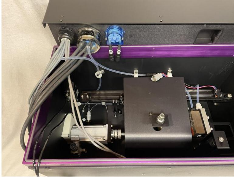
*Figure 47 – Rinse Module – All Cables Disconnected*
