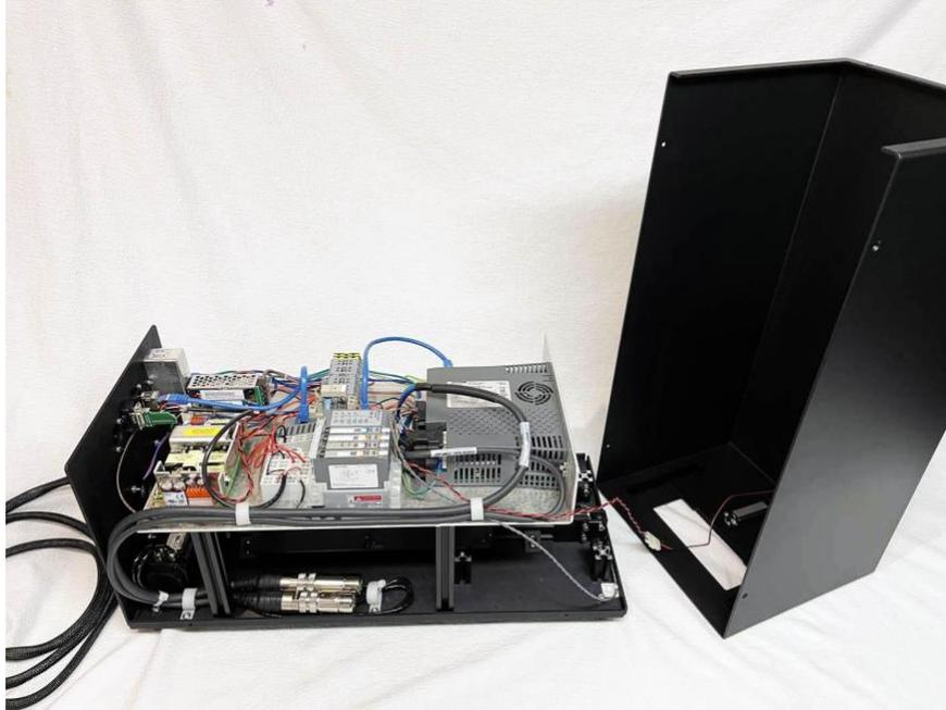
*Figure 65 – Plasma Module – Access to Door Actuator Plug*
