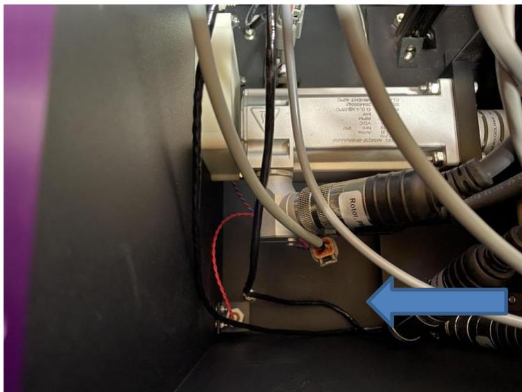
Figure 42 – Rinse Module – Water Level Sensor
