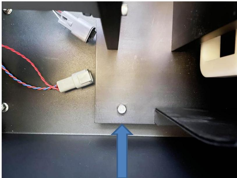
*Figure 53 – Rinse Module – Base Plate 1<sup>st</sup> Nut Location*
