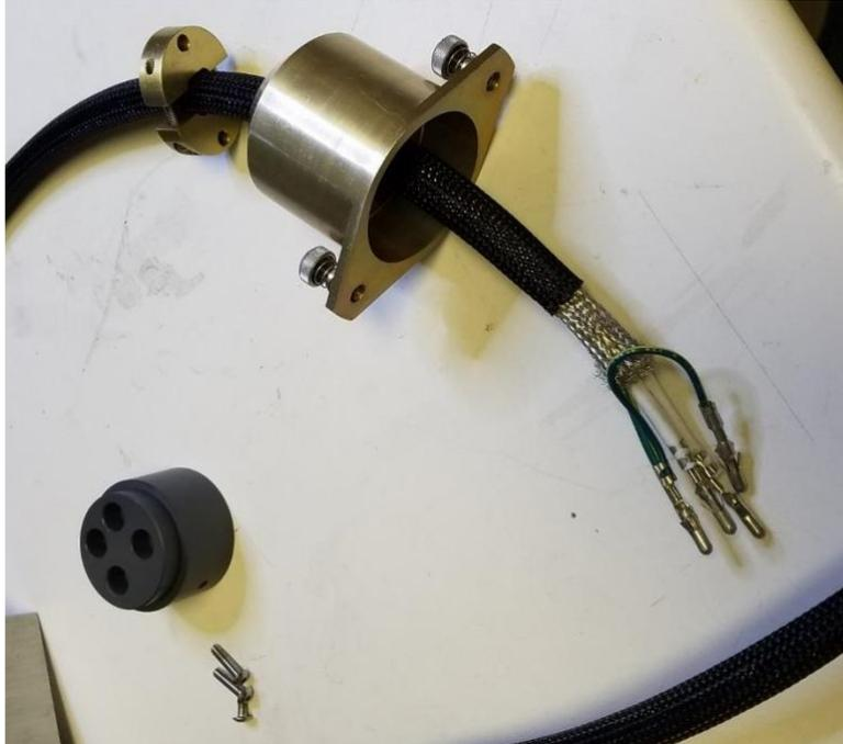
*Figure 70 – Plasma Module – Gold Plug Disassembled*
