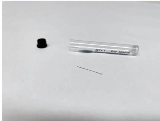
*Figure 16 – Rinse Module Micro Dispense Cleaning Tool*
