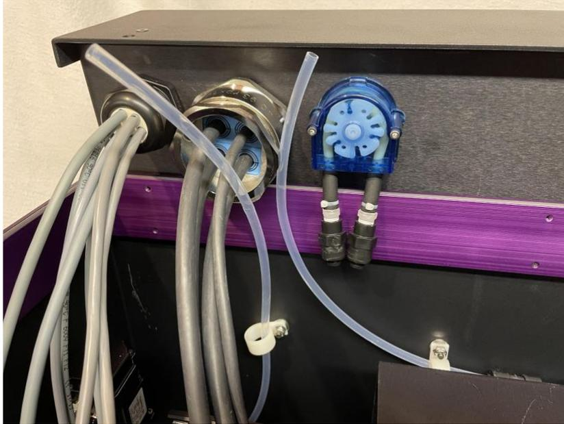
*Figure 39 – Rinse Module – Micro Dispense Tubes*
