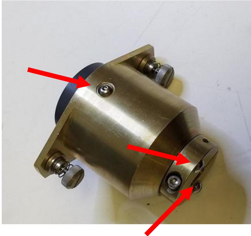
*Figure 71 – Plasma Module – Gold Plug Screw Location*
