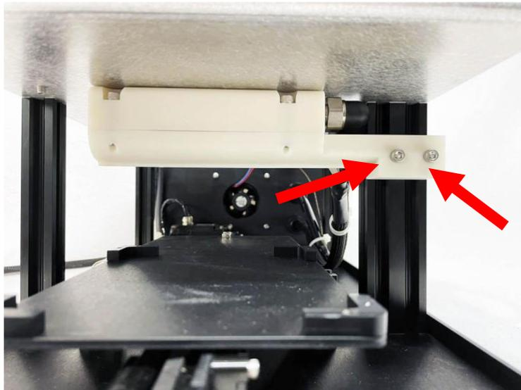
*Figure 68 – Plasma Module – Plasma Generator Screws*
