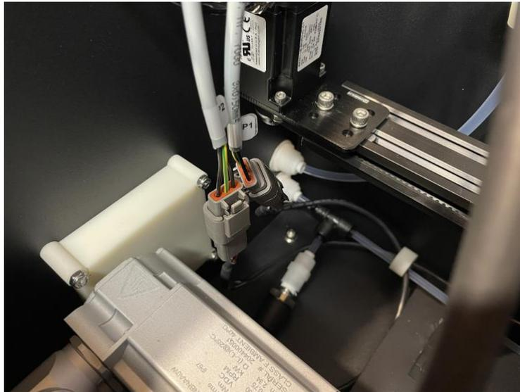
Figure 41 – Rinse Module – Sensor Plugs P1 and P2
