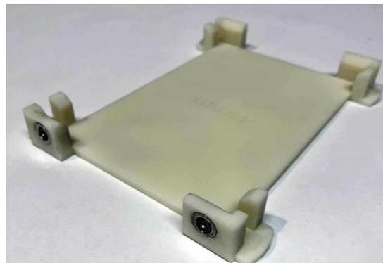
*Figure 11 – Microplate Holder*
