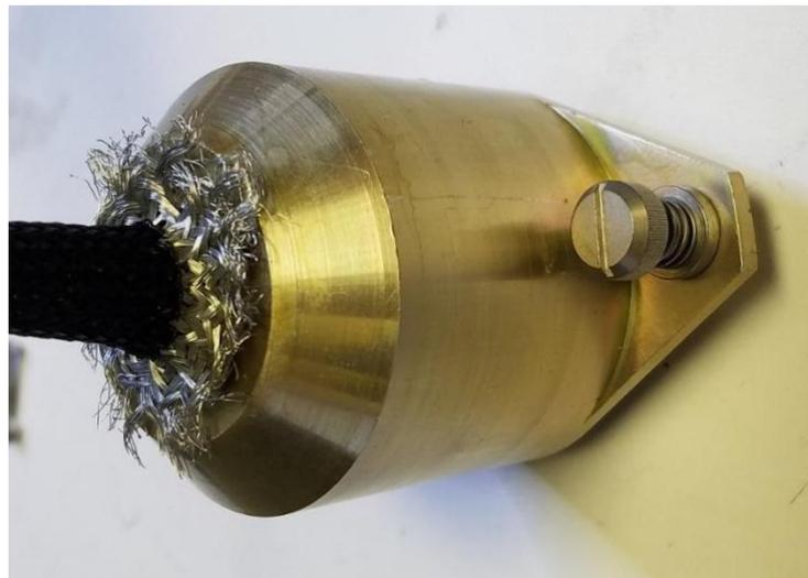
*Figure 77 – Plasma Module – Gold Plug Shielding*
