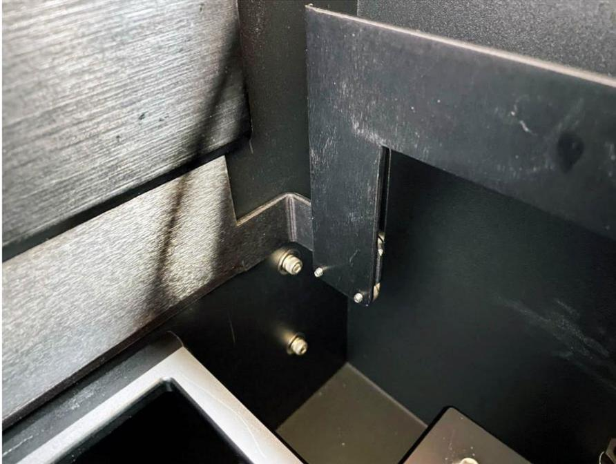
*Figure 49 – Rinse Module – Door Panel (held in place by leaf spring)*
