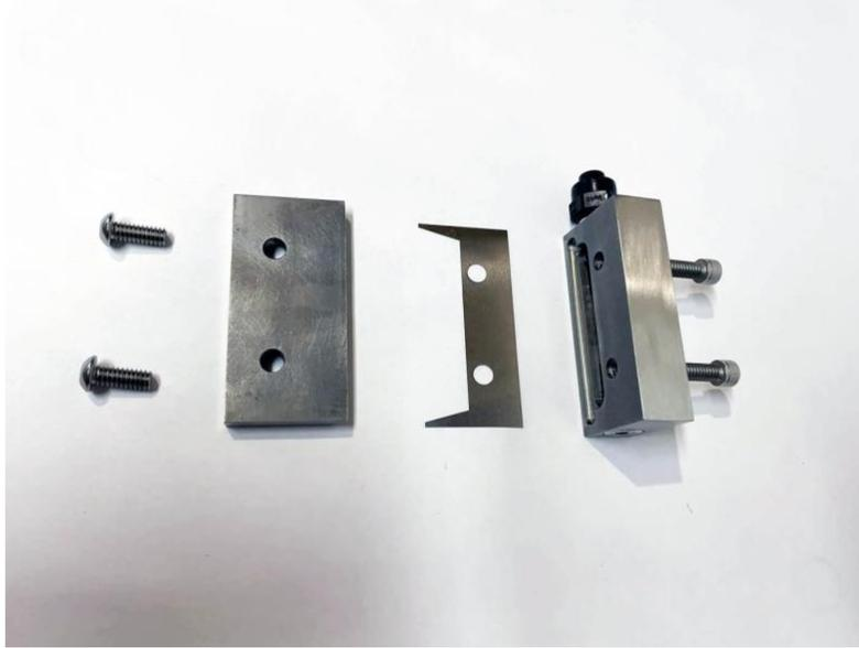
*Figure 81 – Rinse Module – Rinse Head Components*
