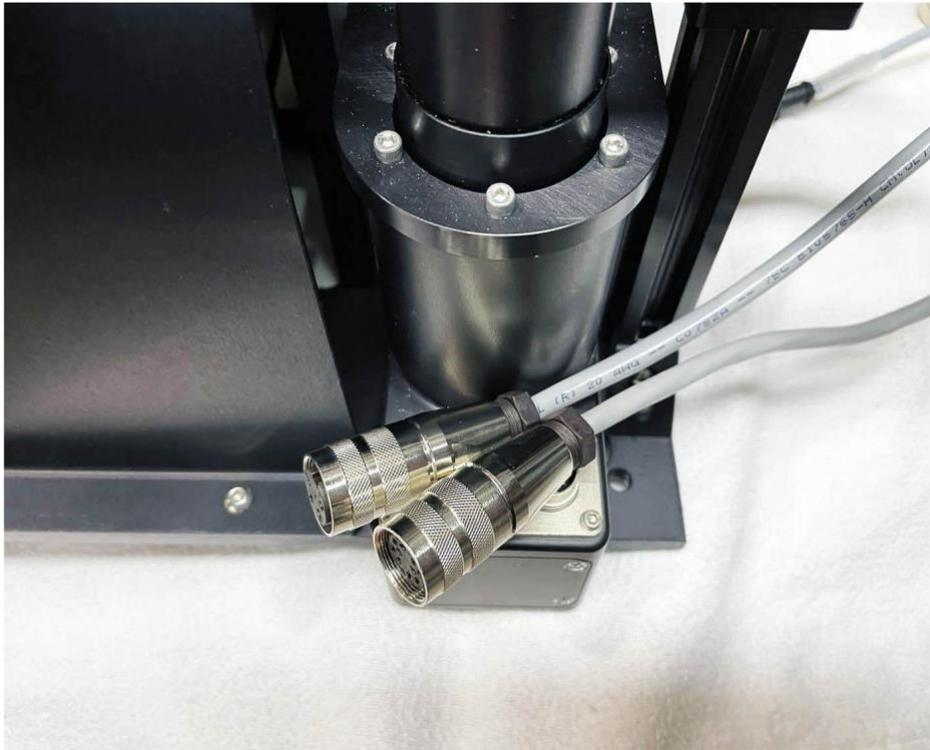
*Figure 62 – Rinse Module – Actuator Plugs Removed*
