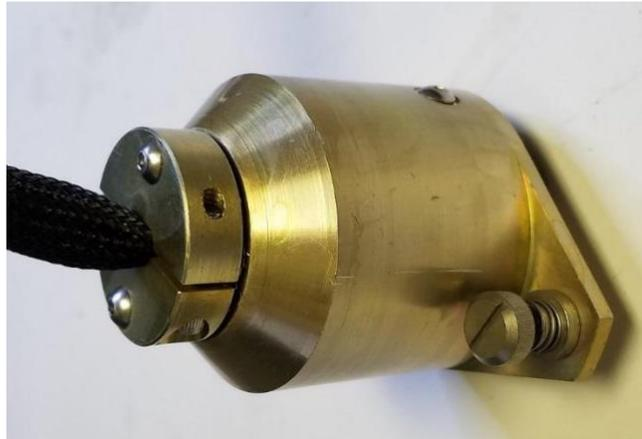
*Figure 78 – Plasma Module – Gold Plug Completed*
