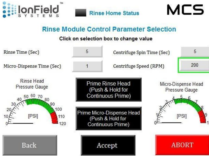
Figure 26 – TOUCHSCREEN – Rinse Module Parameters
