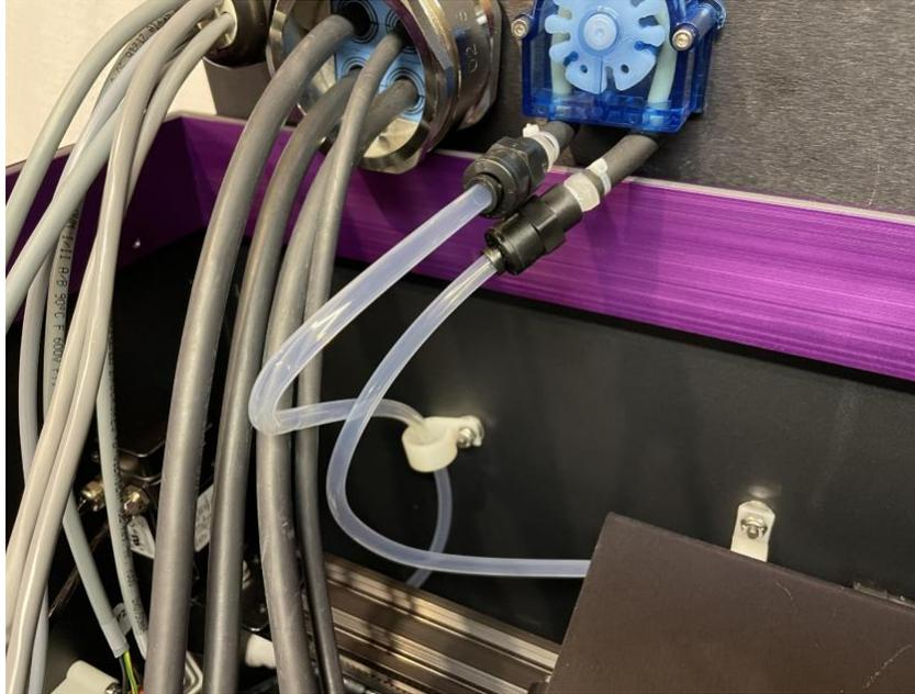
*Figure 37 – Rinse Module – Micro Dispense Tubes*
