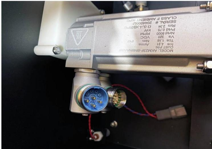
Figure 46 – Rinse Module – Centrifuge Motor Cables Disconnected
