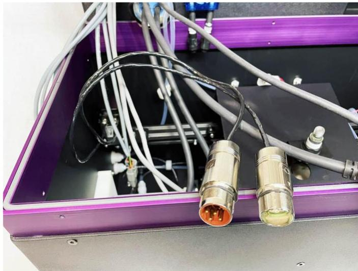
*Figure 44 – Rinse Module – Linear Motor Cables Disconnected*
