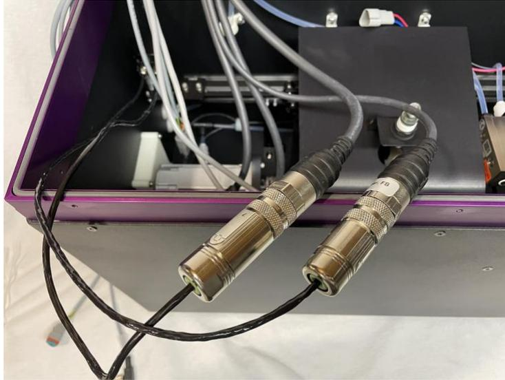
*Figure 43 – Rinse Module – Linear Motor Cables*
