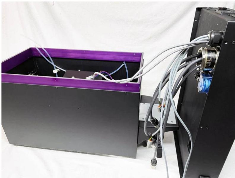
*Figure 48 – Rinse Module – Electronics Lid Removed*
