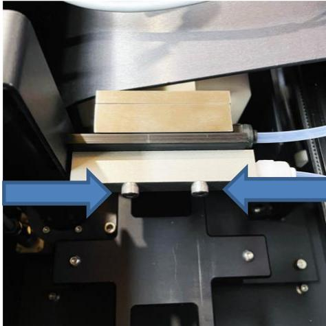
*Figure 84 – Rinse Module – Micro Dispense Screw Locations*
