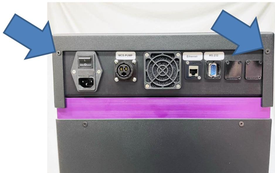
*Figure 33 – Rinse Module - Rear Screw Location*
