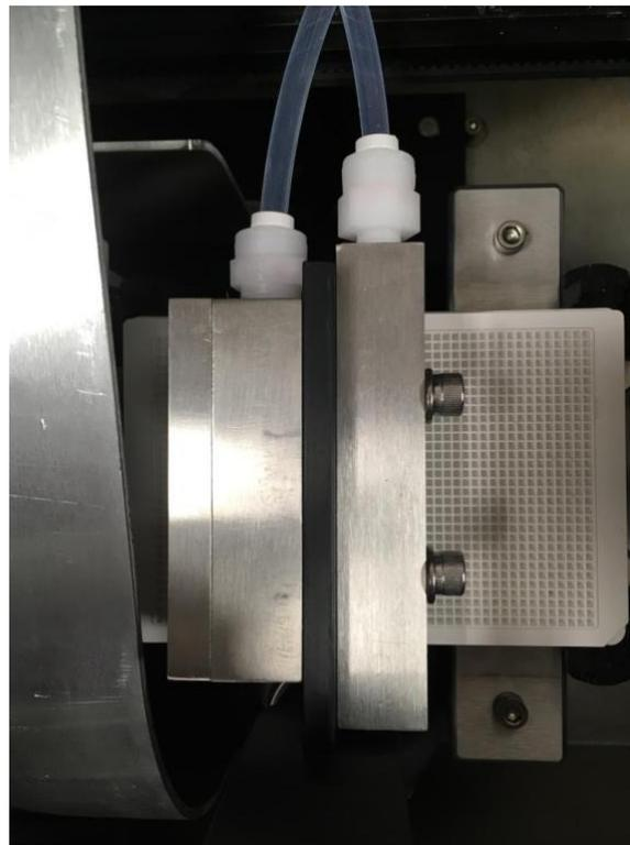
*Figure 87 – Rinse Module – Rinse Head Alignments*
