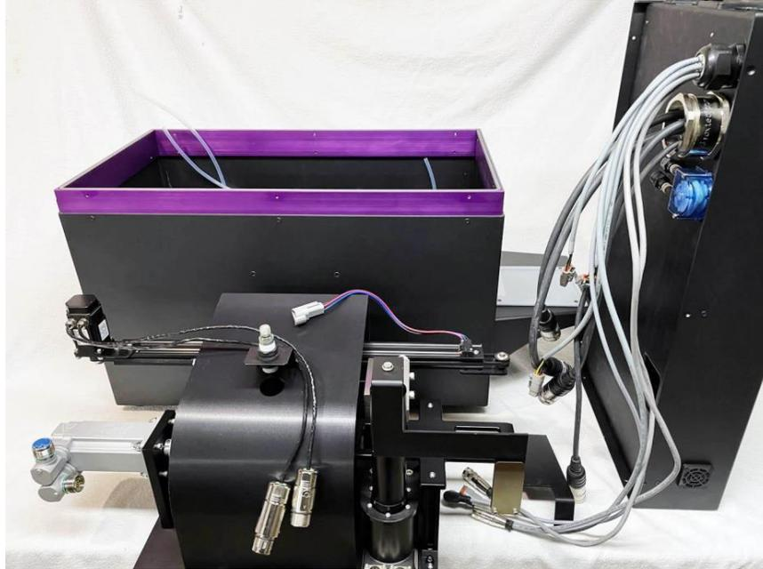
*Figure 60 – Rinse Module – Mechanicals Removed*
