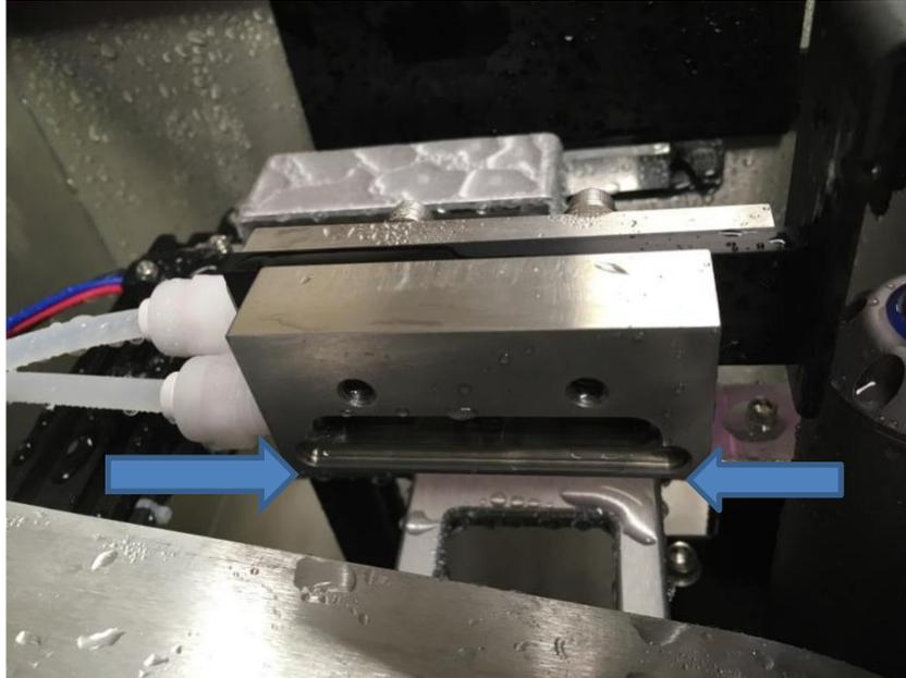
*Figure 80 – Rinse Module – Rinse Head Open for Cleaning*
