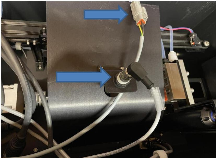
*Figure 40 – Rinse Module – Microplate Sensor and Limit Switch*
