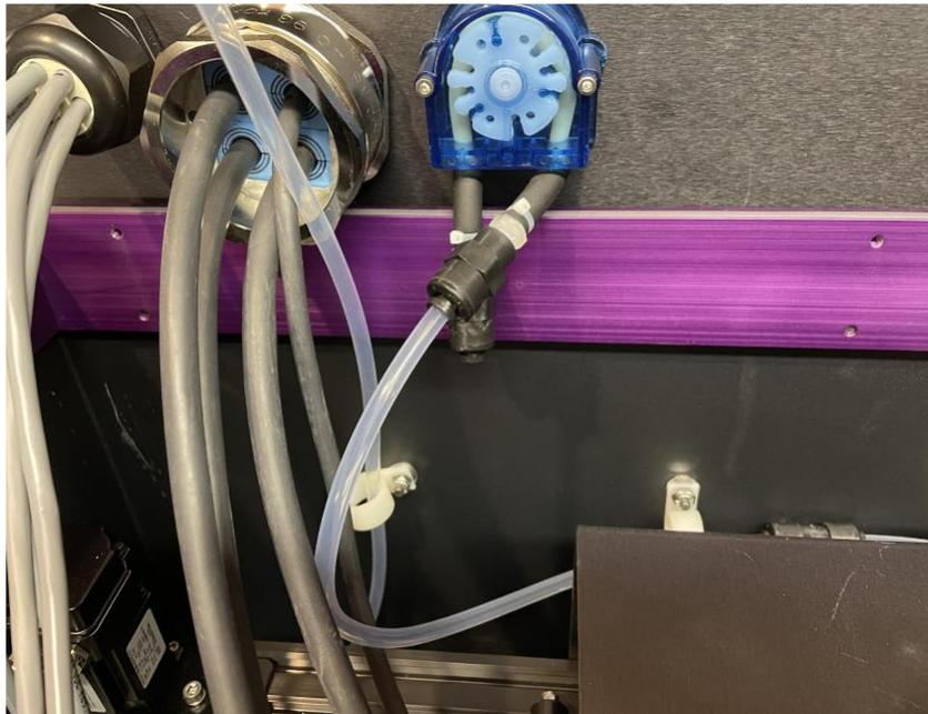
*Figure 38 – Rinse Module – Micro Dispense Tubes*
